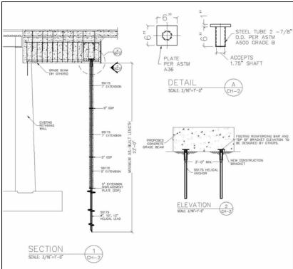
Project Description: East Penn Manufacturing constructed a 24,000 square-foot high-bay battery storage warehouse addition adjacent to two existing buildings. Dual 4ft by 8ft storage racks were to be installed which resulted in floor slab loads in excess of 2000 psf. No additional load could be exerted on an adjacent 17-ft deep basement wall and footing. A special north-south grade beam system and cantilevered exterior wall footing was designed to transfer
